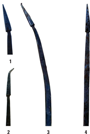
Experimental damage to pila , showing: a bent head caused by attempting to remove a pilum stuck in a shield (1); a bent tip resulting from a deflection (2); a bent shank following treading down a protruding pilum (3) – this took just 1 minute 55 seconds to repair to a serviceable state (4) with a hammer and anvil. (Photos: M.C. Bishop)
